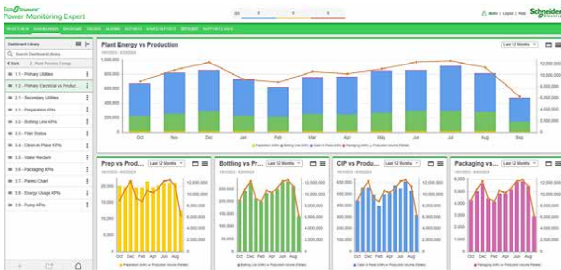
Dashboard dei consumi energetici di produzione, Power Monitoring Expert by Schneider Electric. Production energy consumption dashboard, Power Monitoring Expert by Schneider Electric.
