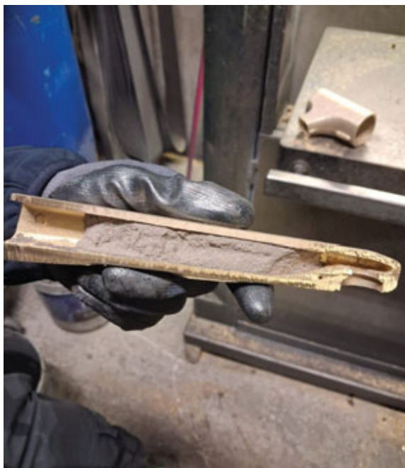
Fig. 5 - Sterratura anima cordis 2K Fig. 5 - Decoring of Cordis 2K core.
