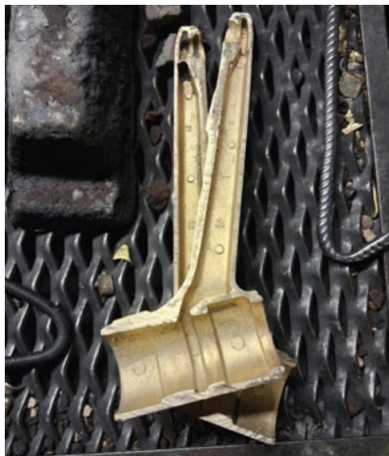
Fig. 6 - Sterratura cordis 3K. Fig. 6 - Decoring of Cordis 3K.
