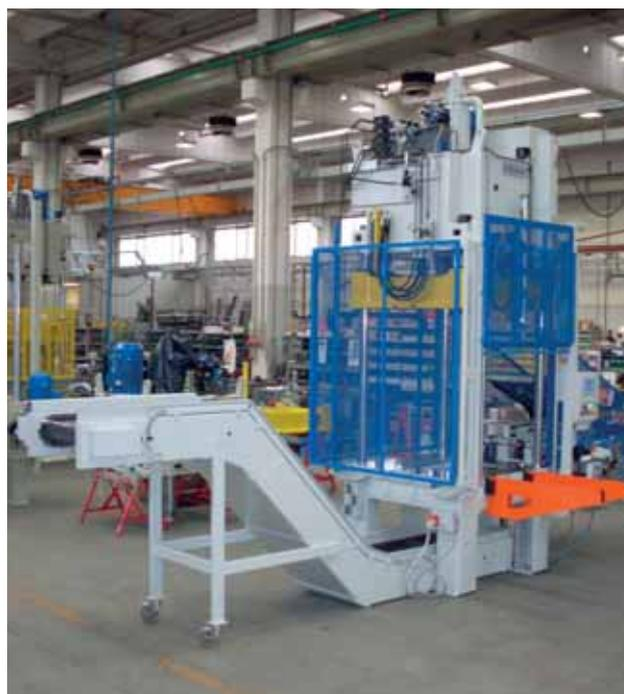
*There is a new player (or, better, it was already present, but always underestimated) in the Die-Casting Automatic Cell: the Trim Technology and its related Trim Process with machinery called "Trim Press" or better "Press for Trimming and Runner Removal". After having been used for a long time in a separate building (a hall made just for that), the Trim Press was finally moved, in a more logistic and efficient way, close to the Di-Casting Machine.*
