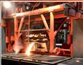
Automatic Pouring Machine P20-W for large size ladle
