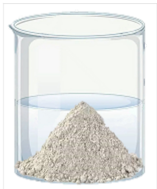
Vetro boro-allumino-silicato ( \phi < 72 \mu\text{m} ) o sodalime ( \phi < 32 \mu\text{m} )
